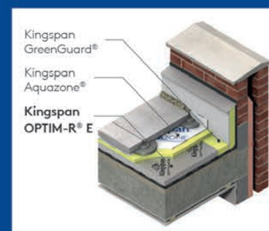
The OPTIM-R® E Inverted Roof System blends high performance OPTIM-R® E with Kingspan GreenGuard®, topped by Aquazone®.
