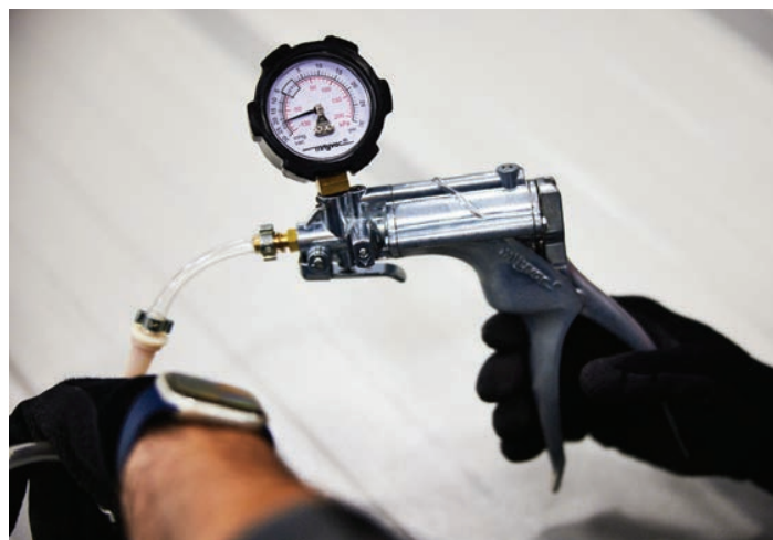
With VACUtest the pressure gauge makes it easy to assess whether the seal is a pass or fail.
