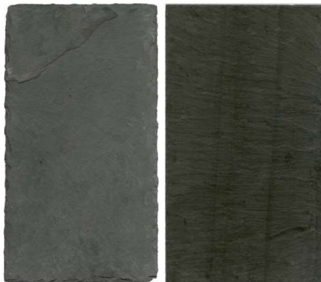
Figure 4. Brazilian material (left), corresponding to IRSC 0, and Spanish roofing slate (right), corresponding to IRSC 1. Lineation (hebra) in this last sample runs north-south. On the other hand, no trace of lineation can be observed in the IRSC 0.
